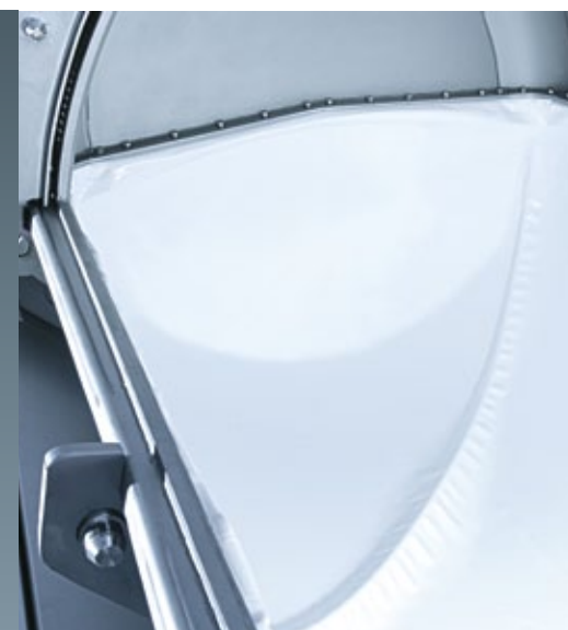
Matching membrane with pomace discharge elements
