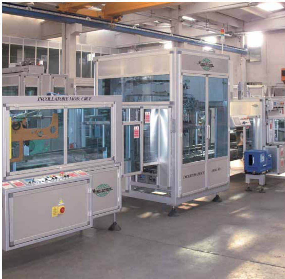
Divisions Inserter. Model 2000/E Suitable to pick-up, open and insert automatically solid carton divisions into cases.
