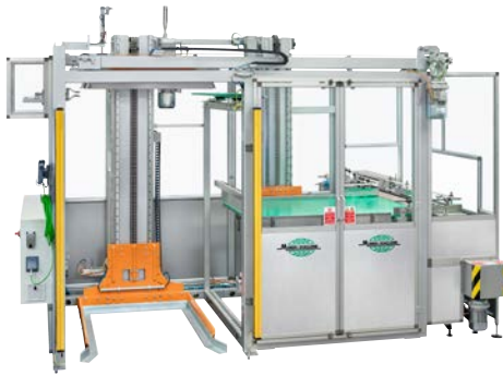
Depalletiser D3 - Sweep off system Machine suitable to depalletise new bottles from pallet with overlapped layers transferring the complete layer with a vertical movement of the pallet.
