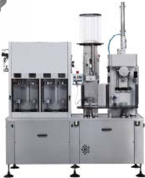
Counter Pressure ISO 6/1/1-A - Automated Monobloc Integrates the operations of; isobaric filling with 6 valves, closure with champagne corks and application of muselets. Different phases and processing times can be set through the electronic operator panel. 750ml - 650/700 BPH, 500ml - 650/750 BPH. 375ml - 800/900 BPH.
