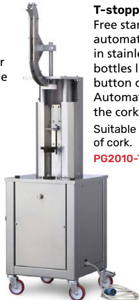
Semi-Automatic Corking Machine Pneumatic bottle lifter. Auto cork distribution by top hopper. Approx 900 BPH. Options: Nitrogen Injection Vacuum Corking. Still Wine: PG2010 Sparkling: PG2010S
