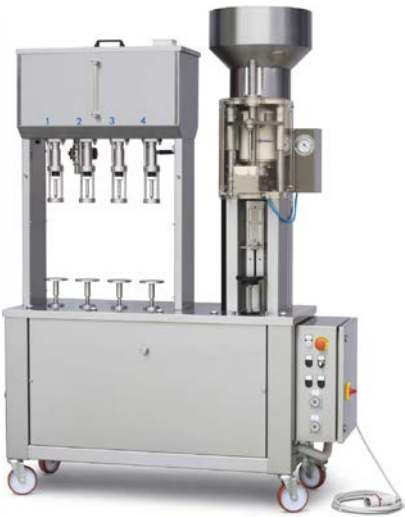
Monoblock Gravity Filler Semi automatic for still wine or spirits. Monoblock with crown, cork or screw capper. 4 valves, drop-down timer, for automatic filling cycle, corker & hopper. PG2010/M
