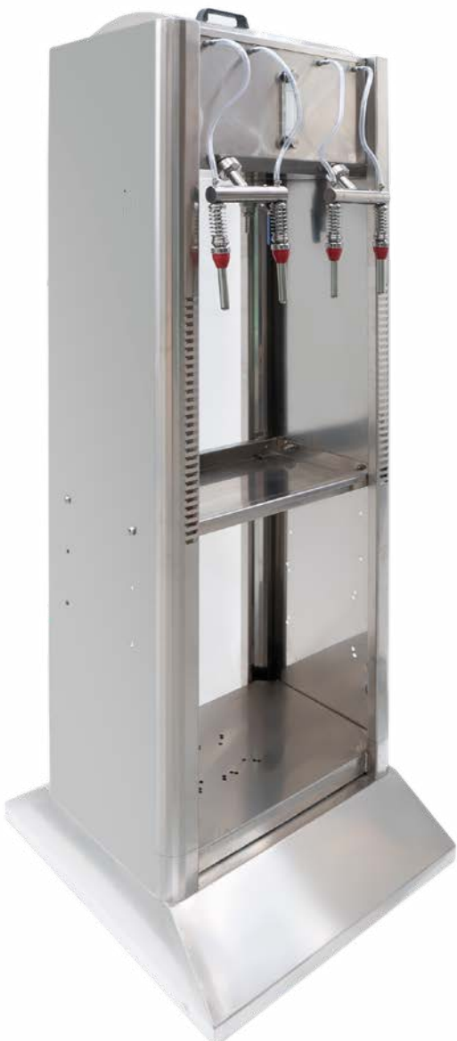
Manual Gravity Bottle Filler 4 or 6 head models available. 500ml to 2L bottles. Articulated nozzles for insertion and removal of bottles. Options: Electric Level Probe, Pump, Plate & Frame Filter. ATEX rating available. MFIL4 / MFIL6
