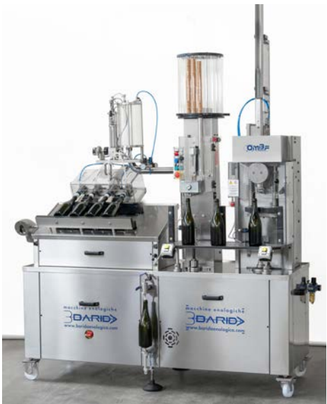
MUIMA TG Auto Monobloc Automatic decrowning assembly, disgorging-dosing-levelling monobloc. Bottles are automatically transferred to the different processing stations. The unit incorporates a corker and wire hooder. Autonomous conveyor. Output approximately 500 BPH.
