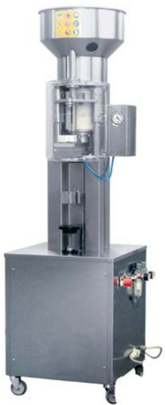
Semi-Automatic Corking Machine Pneumatic bottle lifter. Auto cork distribution by top hopper. Approx 900 BPH. Options: Nitrogen Injection Vacuum Corking. Still Wine: PG2010 Sparkling: PG2010S
