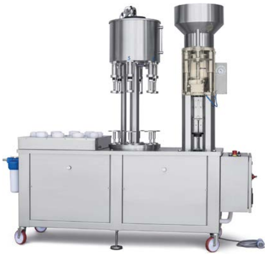
Semi-Automatic Gravity Filling Monoblock 6 valves rotary filler for filling with gravity system, automatic movement, pneumatic bottles lifting. 10 cavity rinser. Mechanical corker machine for T-corks with push button operation and pneumatic bottles lifting. EURO 1061S
