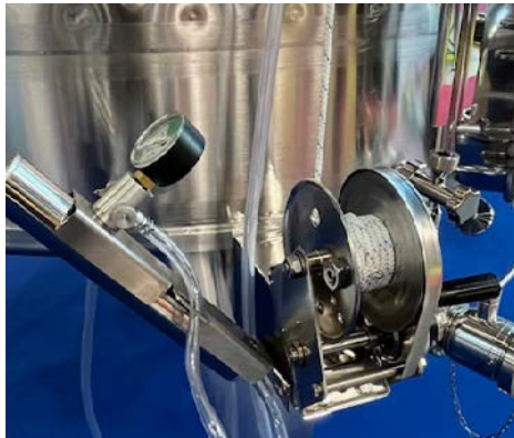
Winch to lift floating lid Plus lid seal pump & pressure gauge
