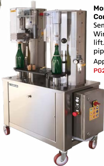
Enolmechanica Multi Function Screw Cap, Crown or Corker The MT-CX Fully auto unit can be supplied in three versions: Screw capper, crown sealer or corker. Can also be supplied as a multi function unit with any two of the three functions listed. 2500 BPH. EMMT+
