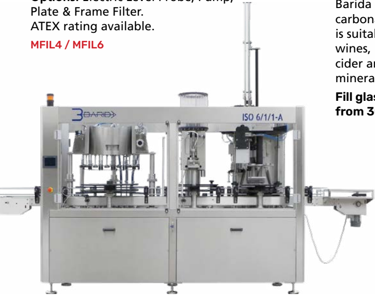
Counter Pressure ISO 6/1/1-A - Automated Monobloc Integrates the operations of; isobaric filling with 6 valves, closure with champagne corks and application of muselets. Different phases and processing times can be set through the electronic operator panel. 750ml - 650/700 BPH, 500ml - 650/750 BPH. 375ml - 800/900 BPH.
