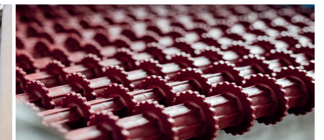
open and closed rollers are separately adjustable in spacing
