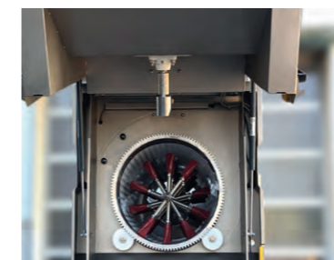
destemming shaft and basket separated, frequency-controlled and adjustable
